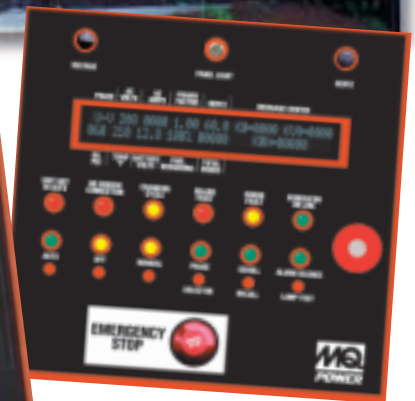
Digital control panel monitors all phases of machine operation.
