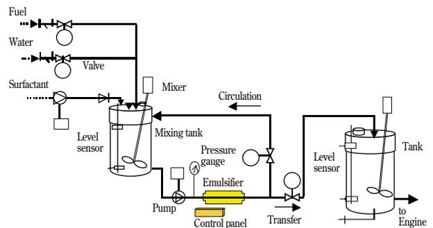
Fig. 3 Fuel Mixing System
