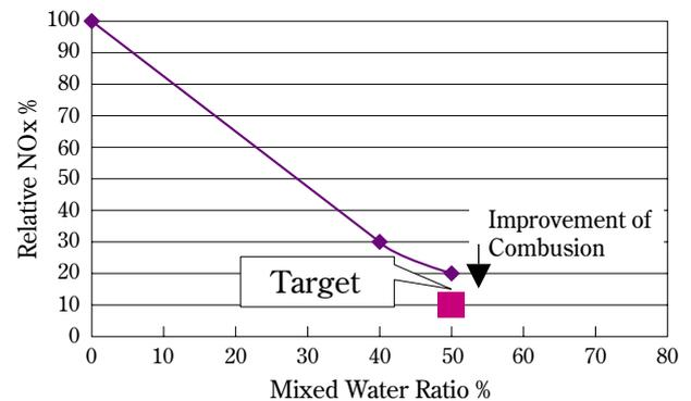
Fig. 9 NOx vs. Mixed Water Ratio
