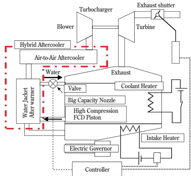
Fig. 7 Engine System
