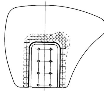
**Fig. 25** Reinforced insert
