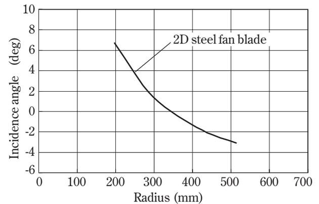
Fig. 6 Two-dimensional fan inlet incidence
