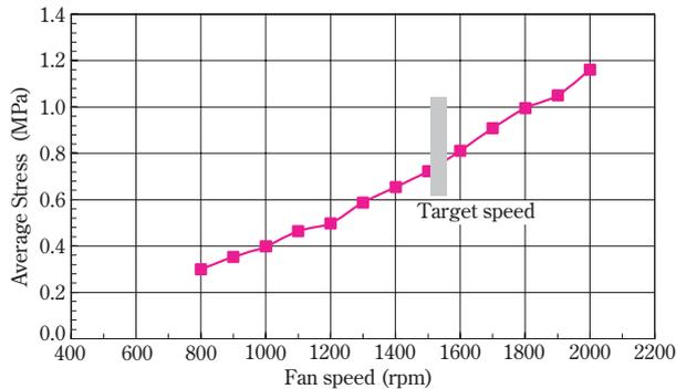
Fig. 27 Average stress (centrifugal stress)
