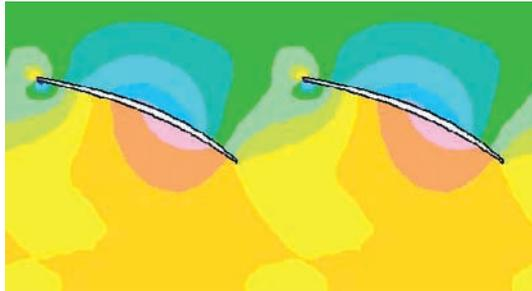
Fig. 19 Pressure distribution of Type1 (860 mm)
