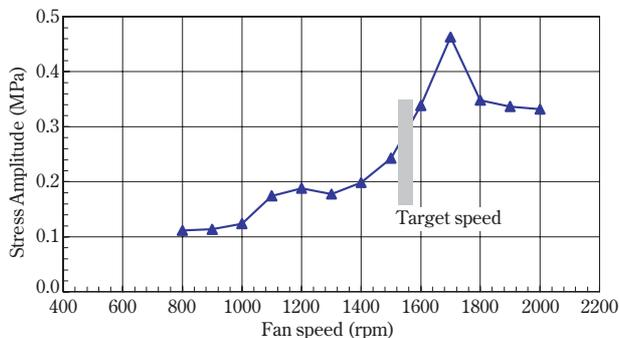
Fig. 28 Fluctuating stress (vibrational component)
