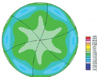
Fig. 21 Front face pressure distribution of Type1
