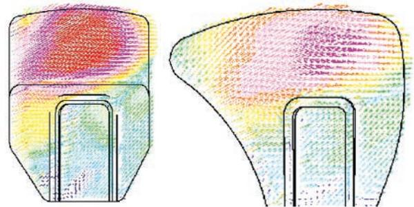
Fig. 16 Blade surface flow of two-dimensional and Type1 fans
