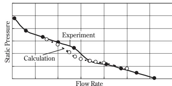
Fig. 12 Comparison with experiment (850 mm hybrid fan)
