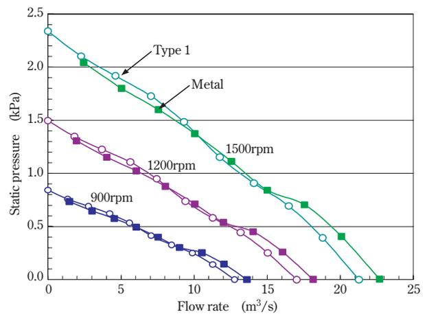
Fig. 22 Flow rate - pressure diagram
