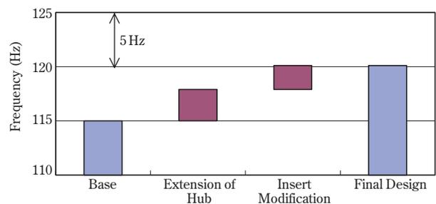
**Fig. 26** Contribution to the increase of first torsional characteristic frequency
