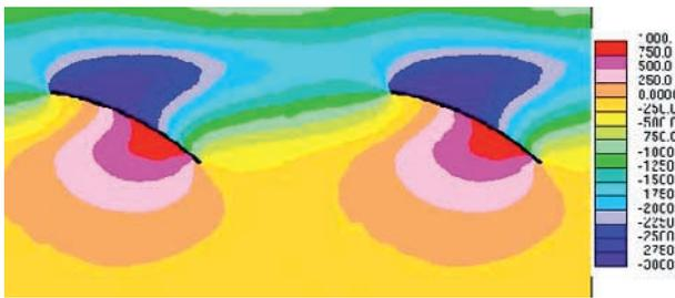
Fig. 13 Pressure distribution of two-dimensional fan (1080 mm)
