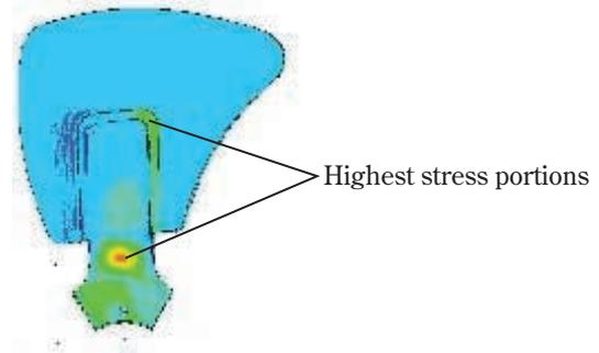
**Fig. 23** Centrifugal stress distribution
