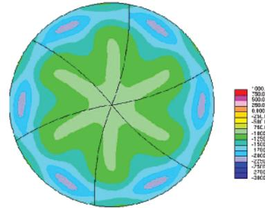
Fig. 8 Front face pressure distribution of steel fan
