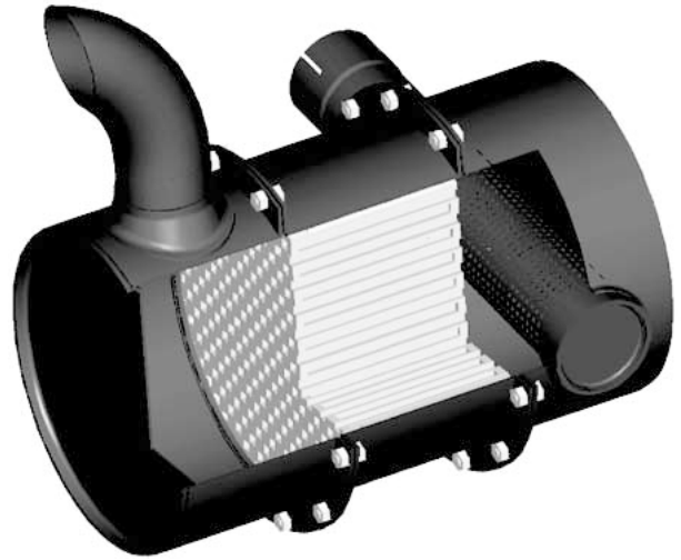
Fig. 12 Cross-sectional view of DPF for PC200 excavator engine
